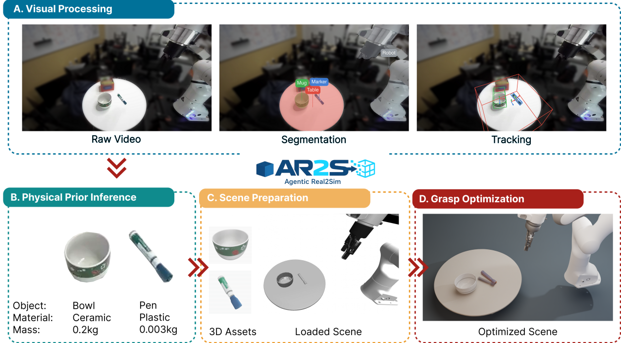
Fig. 1. Agentic Real2Sim architecture. A recorded DROID episode is converted into a simulatable digital twin through four linked agents: The visual processing agent from raw video extracts segmentation and depth masks, geometries and object poses. The physical-prior inference agent attaches object identity, material class, mass hints, and other constitutive properties needed by the simulator. The scene preparation agent initializes a scene with the robot’s initial state, cameras, and reconstructed geometry, and places objects of interest in the correct locations. Simulator-in-the-loop grasp optimization further optimizes object placements to enable successful grasping. The same episode contract supplies the inputs and feedback channels used by the rigid, deformable, and humanoid adapters.
